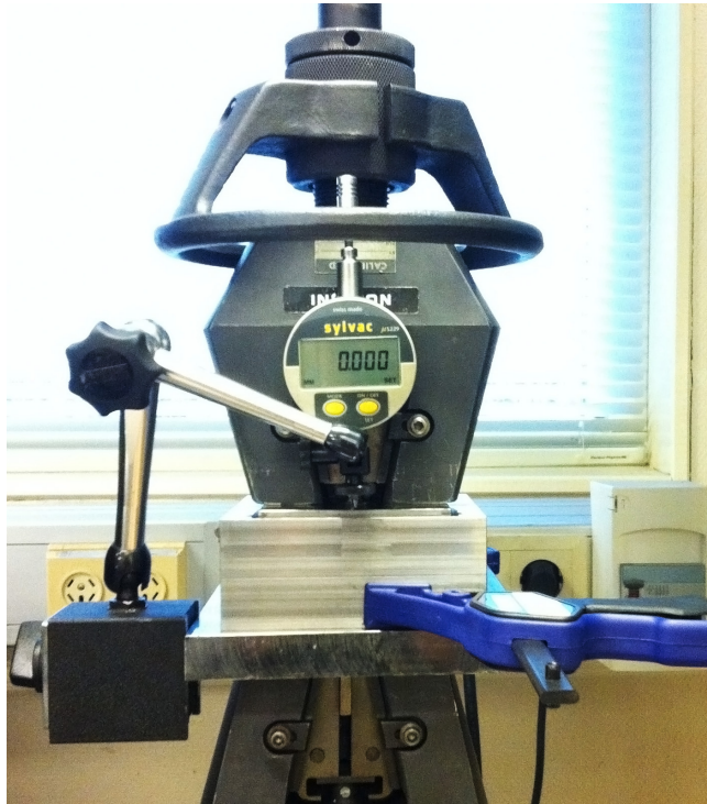
Figure 4.5: The setup of the tensile test. In front one sees the dial that measures the displacement.
