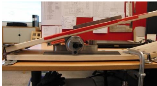
Figure 6.7. Angle of friction test rig
