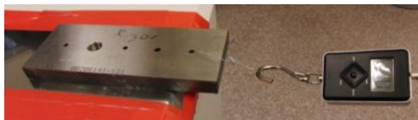
Figure 6.9. Dynamometer test rig
