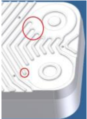
Figure 7.3. Troubling spots on the upper tool
