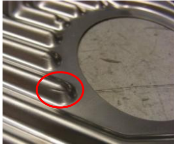
Figure 3.7. Sever thinning that has started to neck
