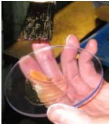
Figure 5. Step 3, Oil applied onto one side of the PVC
