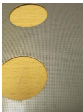
Figure 6.15. Pre printed dots on a raw plate
