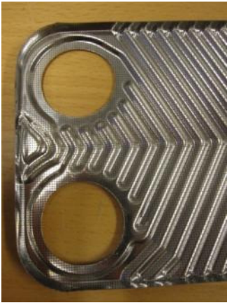
Figure 19. The pressed etched channel
