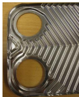
Figure 6.16. Pressed plate with deformed dots
