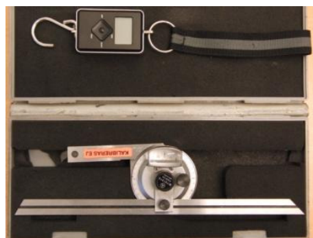
Figure 6.5. Dynamometer (top) and angle ruler (bottom)
