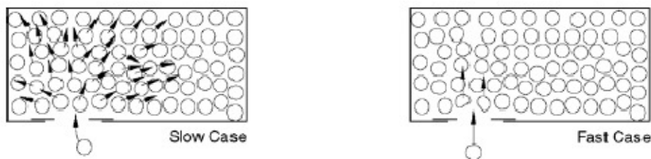
Figure 5.3. Quasi-static elevator example (Quasi-static to the left dynamic to the right) (Getting started with Abaqus)
