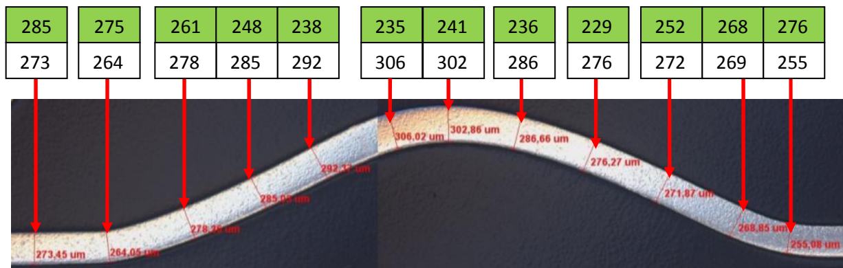
Figure 9.2. Comparison of the 90° cut for the thickness between metallurgy and FEA in \mu\text{m}
