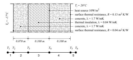
The wall is subdivided into five elements and the one-dimensional spring (analogy) element spring1e is used. Equivalent spring stiffnesses are  $k_i = \lambda A/L$  for thermal conductivity and  $k_i = A/R$  for thermal surface resistance. Corresponding spring stiffnesses per m<sup>2</sup> of the wall are:
