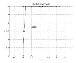
The first eigenmode, 6.98 Hz
