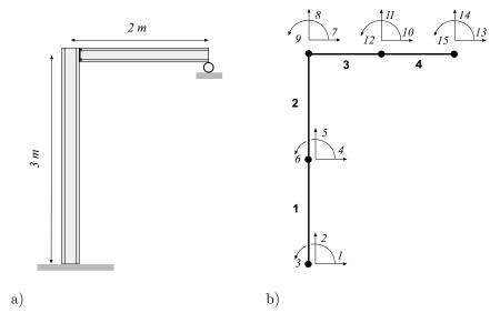
The structure is divided into 4 elements. The numbering of elements and degrees-of-freedom are apparent from the figure. The following .m-file defines the finite element model.
