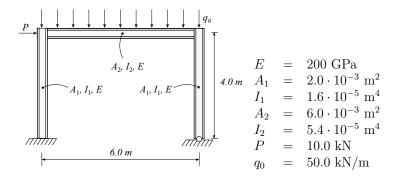
The element model consisting of three beam elements and twelve degrees of freedom is repeated here.
