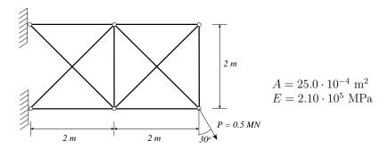
The corresponding finite element model consists of ten elements and twelve degrees of freedom.
