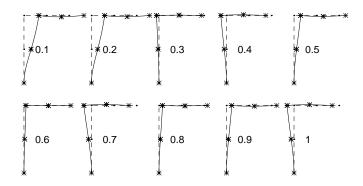
Snapshots of the deformed geometry for every  $0.1~{\rm sec.}$
