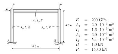
The element model consists of three beam elements and twelve degrees of freedom.
