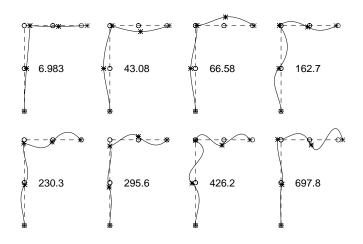
The first eight eigenmodes. Frequencies are given in Hz.
