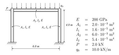
The corresponding finite element model consists of three beam elements and twelve degrees of freedom.
