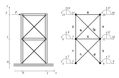
The frame with its coordinates and loading is shown in the left figure, and the finite element model in the right. In the following, the statements for analysing the frame are given as an .m-file.
