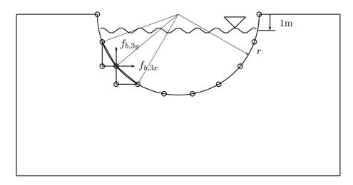
Consider the water channel depicted above. The stresses arising from the water pressure should be analyzed using the finite element method. One step in the finite element procedure consists of calculation of the vector  $\boldsymbol{f}_b$  due to the boundary forces.
