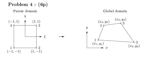
A temperature problem is to be analysed using iso-parametric elements and the approximation for the temperature field within an element is given by
