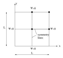
Determine the weak form as well as the FE-formulation associated with the problem. Use the symmetry shown in the figure and define the natural and essential boundary conditions.
