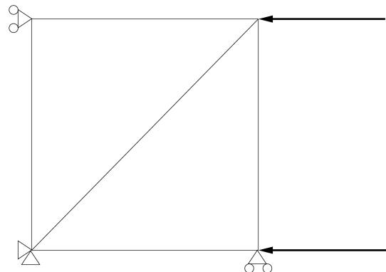
Use the program from E6.1 and E6.2 to calculate the force displacement response. Note as the same element is used and the same geometry the difference in the response is due to the constitutive law. The size of the block above is 10 x10 mm. Use displacement controlled loading.
