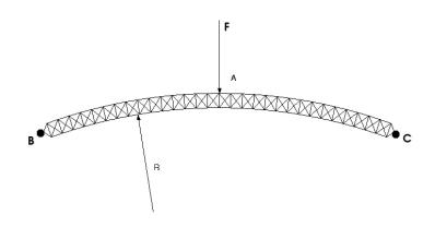
The geometry considered is shown about and is a shallow arch, i.e the same as in E8.1. The task is to determine the dynamic response of the structure. Three node triangle elements are used to define the finite element mesh. Assume that the strain energy for the material is given as in exercise E6.2. The mass density of the material is assumed to equal 7800kg/m<sup>3</sup>. Note that the coordinates defining the geometry is in (mm).
