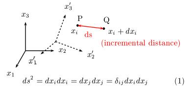
Assumption: length is an invariant (i.e. independent on coordinate system)  $\Rightarrow ds^2 = ds'^2 = dx'_i dx'_i$
