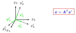
$e_1'$ ,  $e_2'$   $e_3'$  = unit vectors along the  $x_1'$ -,  $x_2'$ - and  $x_3'$ - axis.
