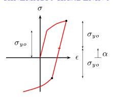
Size of current yield surface is constant = kinematic hardening
