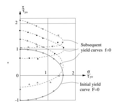
combined torsion and tension tests Ivey (1961)
