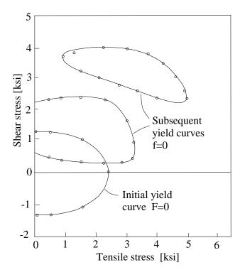
combined torsion and tension tests Phillips and Tang (1972)
