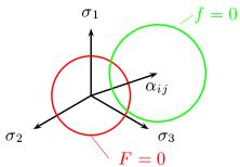
current yield surface moves (kinematic) and expands (isotropic) = mixed hardening
