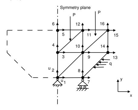
A symmetric structural problem is modelled with 3-node elements and loaded with point loads P and a distributed load q. The right hand side of the structure has 16 degrees of freedom. The matrix relation found from the FE-formulation is given by  $\mathbf{K}\mathbf{a} = \mathbf{f}_b + \mathbf{f}_l$ , where the stiffness matrix is denoted  $\mathbf{K}$ , nodal vector  $\mathbf{a}$ , load vector  $\mathbf{f}_l$  and the boundary vector with  $\mathbf{f}_b$ .
