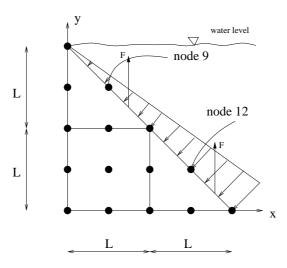
A wall is discretized using two 6 node triangular elements and one 9-node quadrilateral element. The wall is subject to two concentrated loads F applied at (x,y)=(3L/4,5L/4) and (x,y)=(7L/4,L/4). The water pressure is perpendicular to the boundary and given by  $p = \rho gh$ , where h represents the depth.
