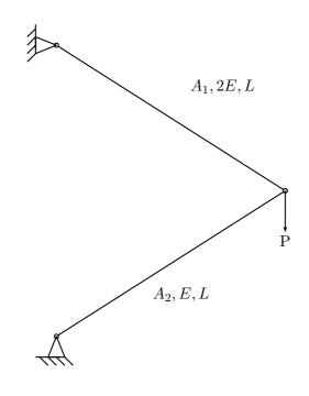
Find the optimal stiffness for the constraints  $|A_i| \leq V_o/2L$  and the volume  $V \leq V_o$ . The design variables in the optimization are the cross section areas,  $A_i$ . The vertical distance between the supports is L. Use Lagrangian duality.
