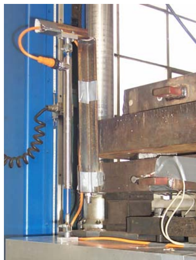
Figure 7.4. The displacement transducer.
