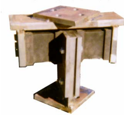
Figure 5.3. Test rig for the dampers.
