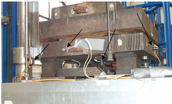
Figure 7.3. The arrangement of four accelerometers on the mass (marked with arrows). The displacement transducer is located to the left in the picture.
