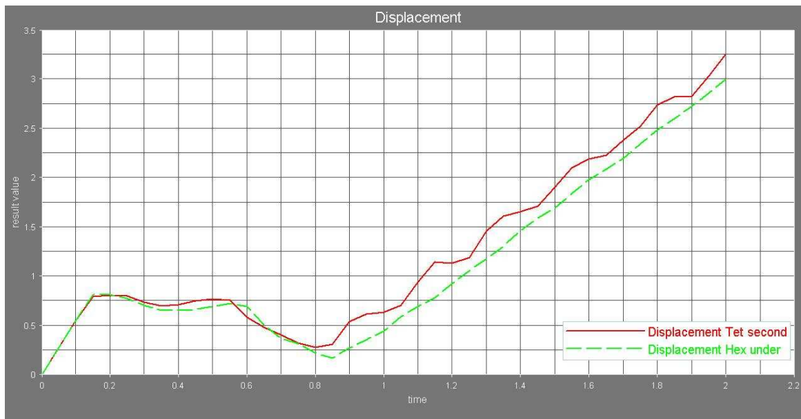
Figure 8.8: Displacement for simulations in Abaqus. Solid line correspond to model using tetrahedron elements and dashed line correspond to model using under integrated hexagon elements.
