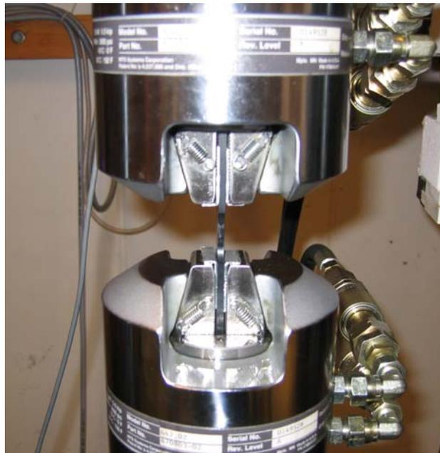
Figure 5.5: MTS tensile testing machine.
