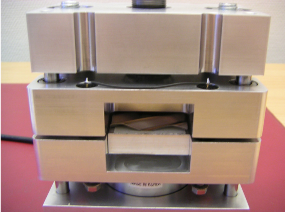
Figure 5.2: Compression device with the plate and gasket inserted.
