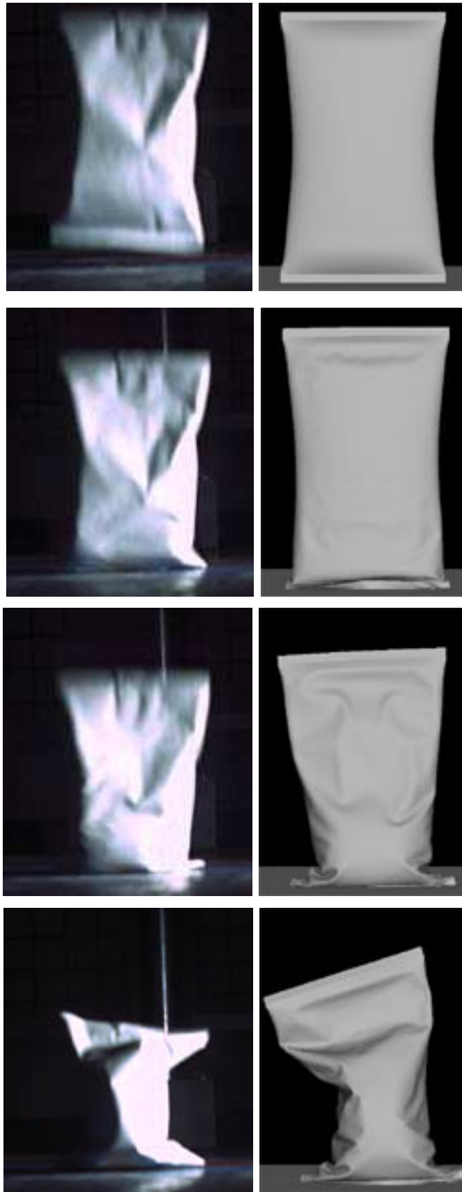
Figure B.3: Comparing vertical falls in a side view.
