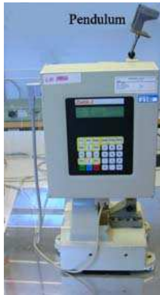
Figure 5.3: Dynamic pendulum test equipment.
