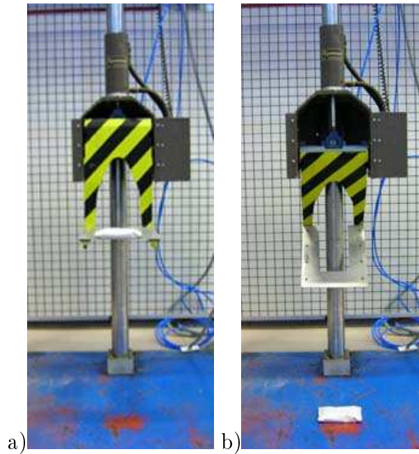
Figure 5.1: Drop test equipment a) initial position and b) final position.
