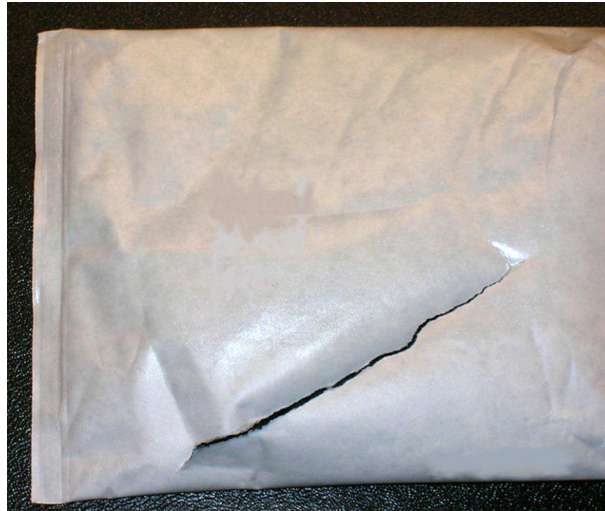
Figure 5.2: A material crack in a package.
